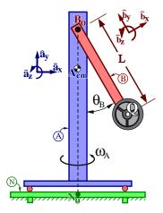
Complete the MG road-map for the turntable's "spin-rate"  $\omega_A$  (Note: The "about point" is not unique)
