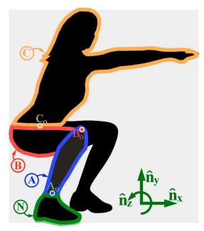
An inefficient way to form equations for  $T_A$ ,  $T_B$ ,  $T_C$  is to use the Newton/Euler equations and **free-body diagrams** (FBDs) for each of A, B, C. For a 3D analysis, this "brute force" technique requires 15 equations and 15 unknowns, and even a 2D analysis, requires 9 equations and 9 unknowns.
