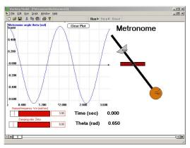
To answer each question with Working Model, click the **Reset** button (if necessary) and click and drag the sliders that control the numerical values for  $\omega_n$  (measured in rad/sec) and  $\zeta$  (dimensionless). To start the simulation, click the **Run** button, and to stop it, click the **Stopil** button.
