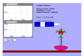
To begin, double-click on the file HarmonicForcingPogoStick.wm2d. To answer each question with Working Model, click the Reset button (if necessary) and click and drag the slider that controls  $\Omega/\omega_n$  (the ratio of the forcing frequency to the system's natural frequency). To start the simulation, click the Run button, and to stop it, click the Stop button.
