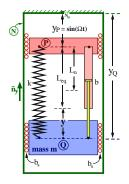
(a) Complete the following sketches. Note: y(t) characterizes how Q moves relative to P and  $y_Q(t) \triangleq y_P(t) + y(t)$  characterizes how Q moves relative to N.
