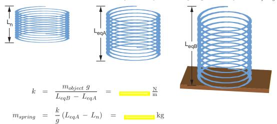
• Calculate the motion's **natural frequency**  $\omega_n$  and  $\tau_{\text{period}_{analytical}}$  (the mathematically determined **period of vibration**).
